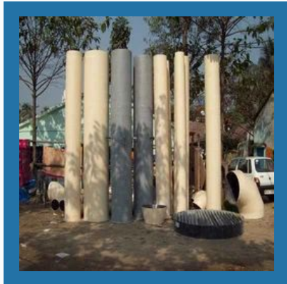
Acid Fume Exhaust Ducts
