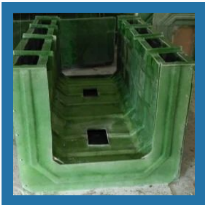
FRP Mould for RCC Gutters Casting
