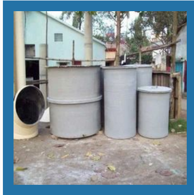
Acid Dosing Tanks
